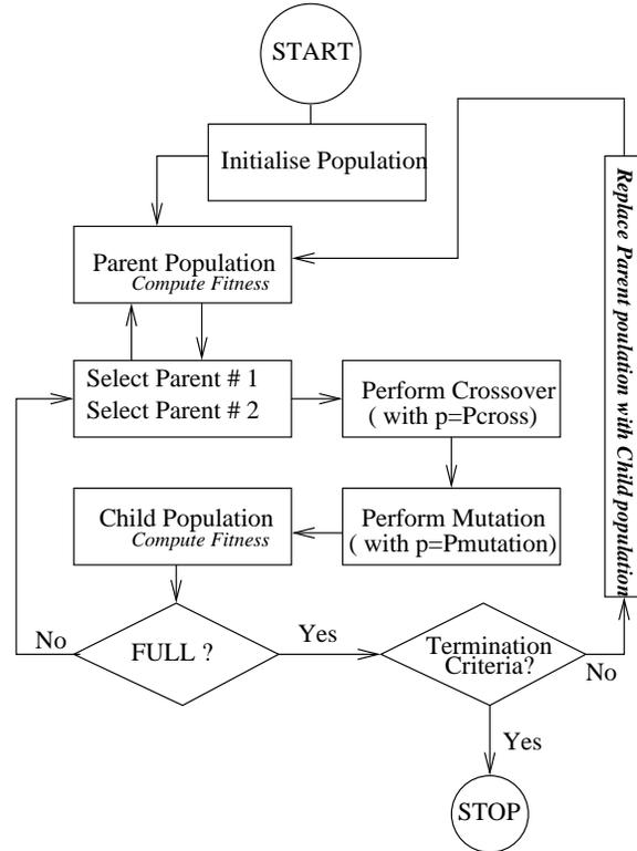
Fig. 3. Block diagram of the Genetic Algorithm
