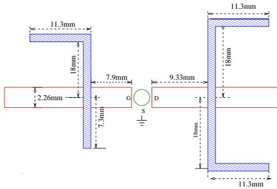
Fig. 4. Slot matched microwave transistor amplifier.
