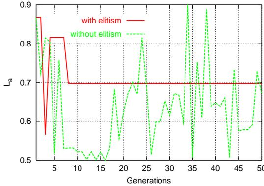
Fig.8. Variation in the slot parameter  $L_a$  as a function of the generation number, with and without elitism.
