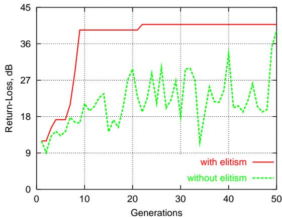
Fig. 9. Return Loss characteristics of the synthesized antenna as a function of the generation number.
