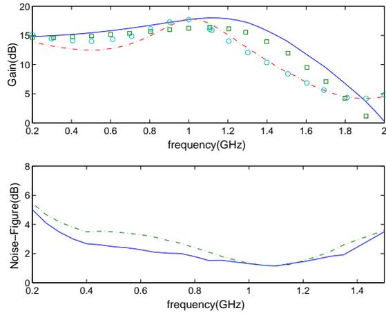
Fig. 5. Gain and noise figure characteristics of a slot matched microwave transistor amplifier.
