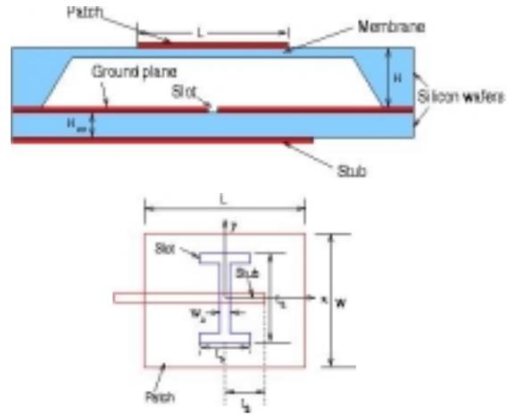
Fig. 6. Side and top view of a silicon micromachined H-slot coupled patch antenna.
