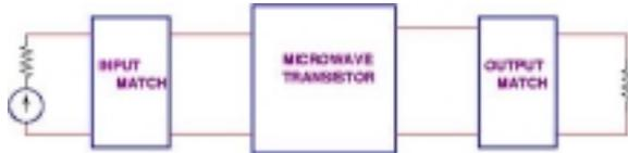
Fig. 2. A microwave amplifier where the input and output match sections is shown separately.
