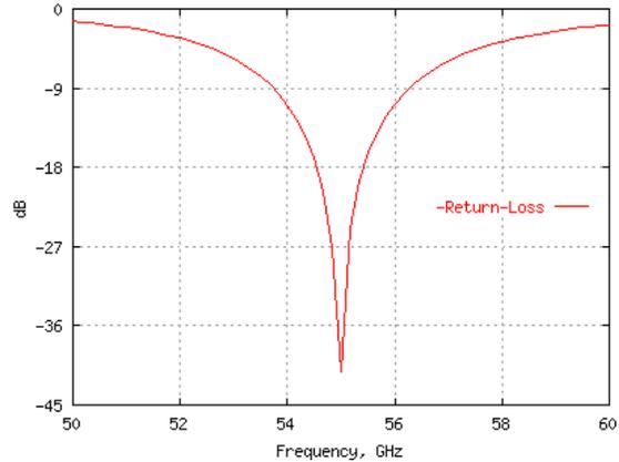
Fig.10. Return loss characteristic of the synthesised antenna as a function of frequency.
